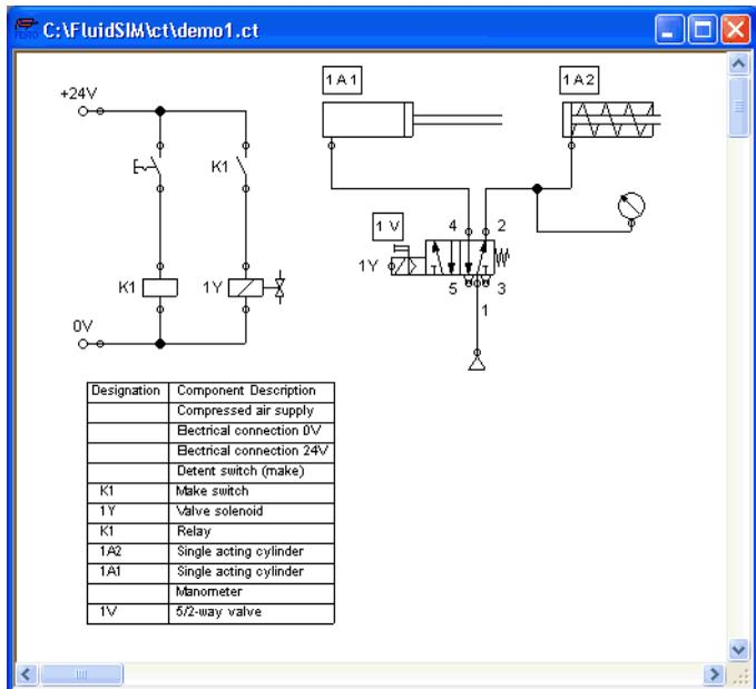
The screenshot displays the FluidSIM software window titled "C:\FluidSIM\ct\demo1.ct". The main area shows a complex circuit diagram with various components labeled: +24V, 0V, K1, 1Y, 1A1, 1A2, and 1V. The circuit includes a 24V power source, a switch (K1), a valve solenoid (1Y), a relay (K1), a manometer (1A1), a single acting cylinder (1A2), and a 5/2-way valve (1V). A parts list table is located at the bottom of the window, listing the components and their descriptions.
