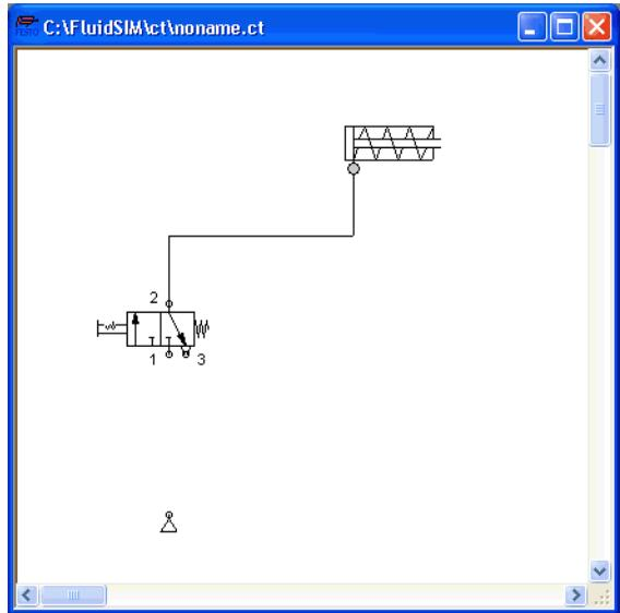
FluidSIM automatically draws a line between the two chosen connections. The mouse cursor changes to the prohibited sign
