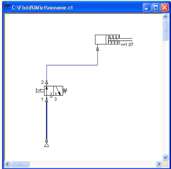
After the cylinder has been extended, the pressure in the cylinder supply line must inevitably increase. This situation is recognized by FluidSIM and the parameters are recalculated; the pressure at the compressed air supply increases to the preset operating pressure.
