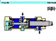
This design features the characteristics of two double acting cylinders forming a single unit. This increases the effective piston area of the unit for high force applications. It is suitable for applications where a large force is required but the cylinder diameter is restricted.
