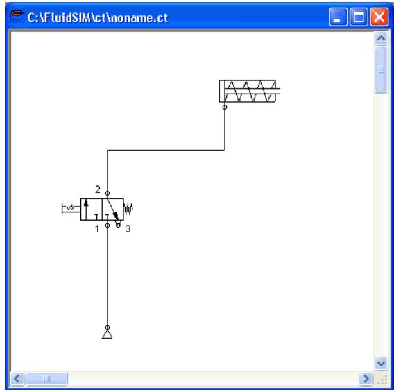
The circuit diagram has been completely drawn and connected. Attempt to simulate this circuit.
