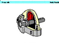
The rotary actuator is compact with high torque ratings. The force is transmitted to the drive shaft by a rotary vane. The range of angular movement is adjustable with end stops. The angle can be adjusted between 0° and 180°.
