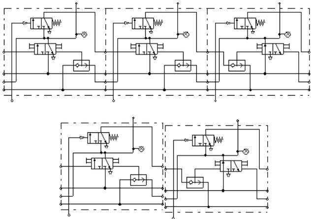
This concept of an automatic component linking is not restricted to stepper modules only; in fact, automatic component linking applies whenever connections of the same type overlap.
