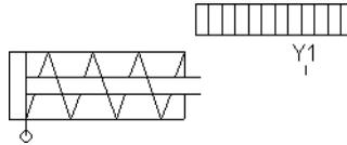
As a consequence, the cylinder will activate the switch or the valve labeled "Y1" if its piston has traveled by 35 mm. To define a label in the electrical circuit double click on the respective component; to define a label at a mechanical actuator of a valve double click the respective "connection" of the valve.
