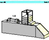
**Problem:** A cylinder is used to transfer parts from a magazine. If either a push-button or a foot pedal is operated, then the cylinder is to advance. Once the cylinder has fully advanced, it is to retract to the initial position. A 3/2 way roller lever valve is to be used to detect forward end position of the cylinder.
