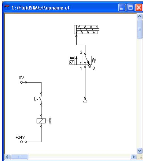
So that the valve can be controlled by the solenoid, you have to link the components with a label.
