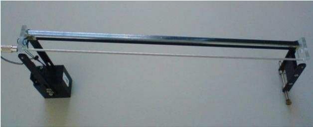
Figura 5-1 Módulo Esfera y Viga (Ball and Beam)
